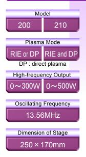
Purpose : Removal of Organic films, Surface cleaning, Surface reforming, Surface etching etc.
